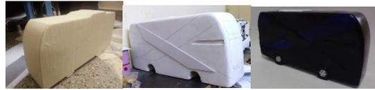
Fig 7: Scale down appearance model (exterior)
