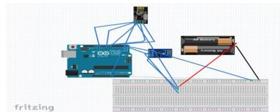
**Fig. 5 Circuit Connection of Receiving Unit on the Breadboard**
