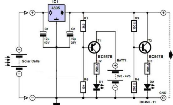
Fig. 8 Solar cell voltage regulator circuit diagram
