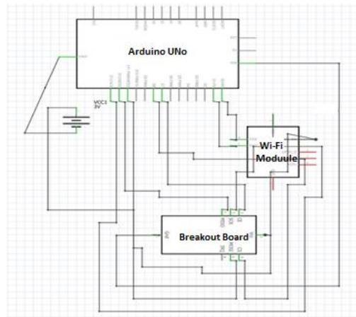
**Fig.4 Circuit Diagram for the Receiving Unit**
