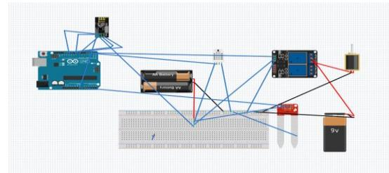
**Fig. 3 Circuit Connection of Control Unit on the Breadboard**
