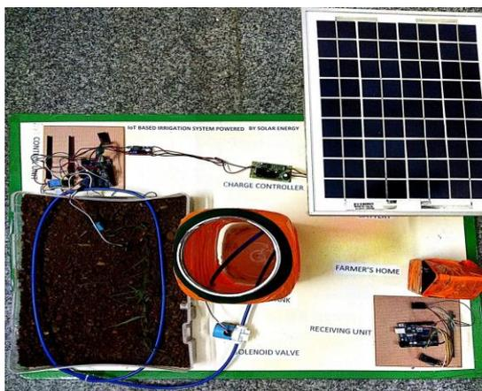
Fig. 7 Experimental setup of proposed system
