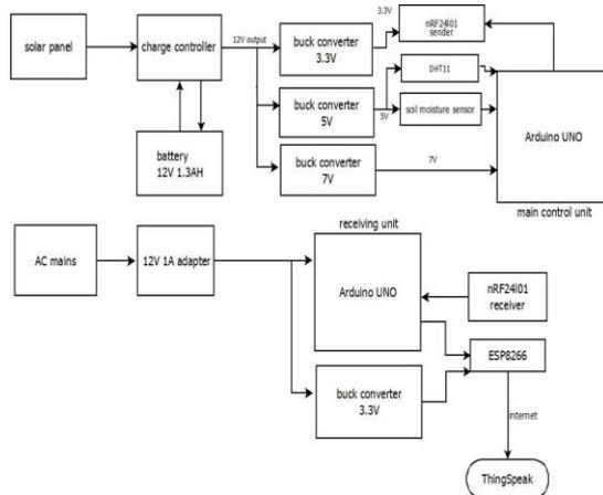
**Fig. 1 Architecture of the proposed design**
