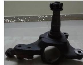
Fig.1 Steering Knuckle Assembly
