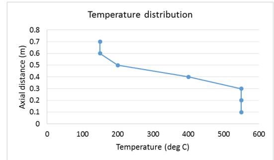
**Fig. 4 Temperature distribution updraft gasifier showing the temperature zones**
