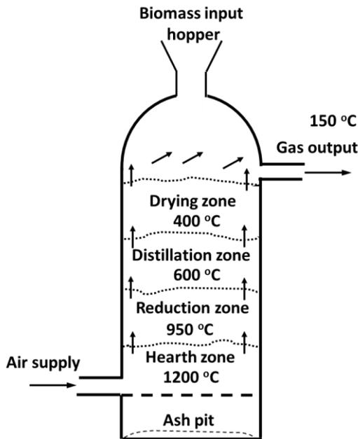
Fig. 1 Schematic of a typical updraft gasifier showing the temperature zones
