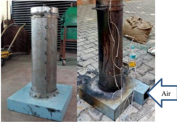
**Fig. 2 Fabricated gasifier setup showing the cylindrical reactor, rectangular base with air inlet**
