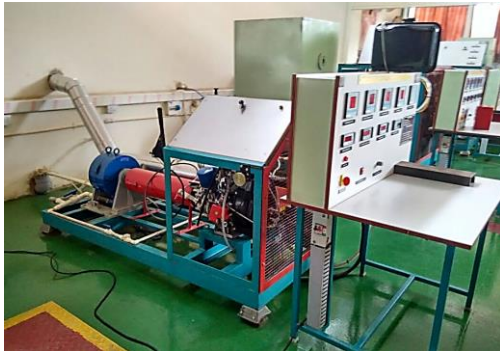
Fig. 3 Engine test rig
