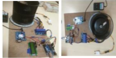
Fig. 5 Experimental setup using GSM and Bluetooth
