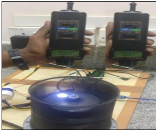
Fig. 8 Real time motor speed measurement using tachometer
