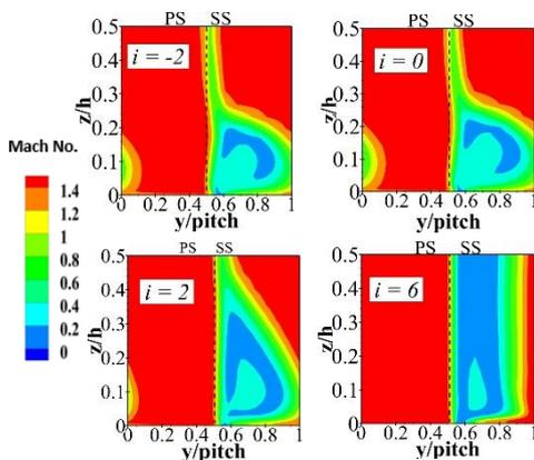
Fig. 7 Mach number distribution on streamwise Plane-A at different incidence angles
