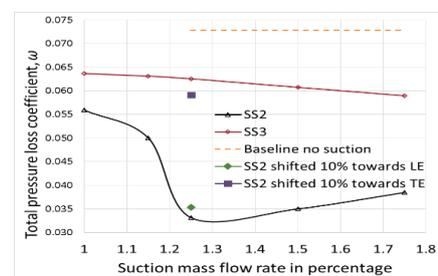
Fig.9 Variation of  $\omega$  with  $m_{suc}$  at  $i = -2^\circ$
