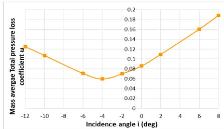
Fig.6 Total pressure loss coefficient at streamwise Plane-A
