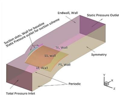
**Fig.1 Cascade geometry and boundary conditions**
