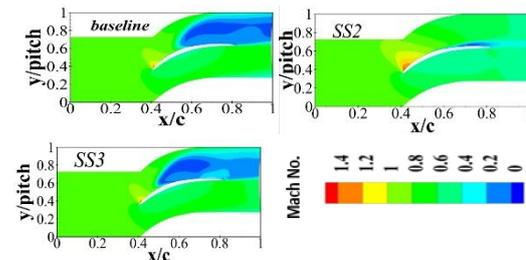
**Fig.12 Mach number contours on pitchwise Plane-B at  $z/h=0.05$ ,  $m_{suc} = 1.25\%$**
