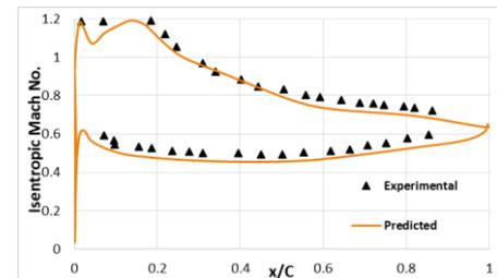
**Fig. 5 Isentropic surface Mach number distribution on blade at mid-span under design conditions**
