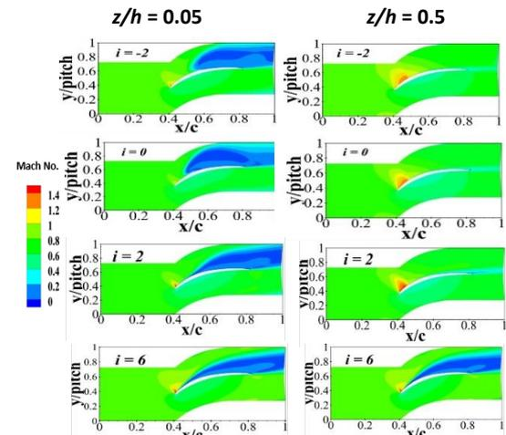
Fig. 8 Mach number distribution on pitchwise Plane-B and C at different incidence angles
