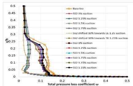
**Fig.10 Total pressure loss coefficient along the span at streamwise Plane-A**
