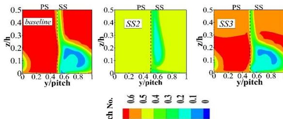
**Fig.11 Mach number contours along half blade span on streamwise Plane-A,  $m_{suc} = 1.25\%$**
